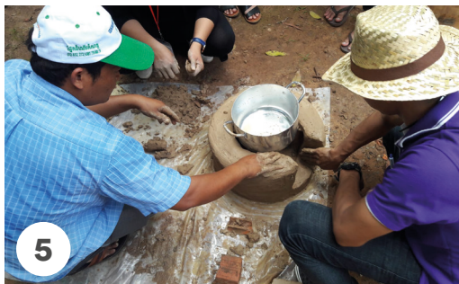
5 Finalise the hole where wood is added from. Wood can be added without lifting the pot off the fire. Different models of the stove can have different styles of holes (see pictures 5B and 6).
